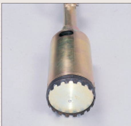
Drilling-crown, extruder in lower position
