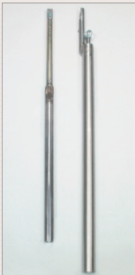
Gouge auger and piston sampler
