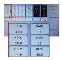
Elevated humidity condition with the equilibrator in saturated foam in the same dry ambient condition
