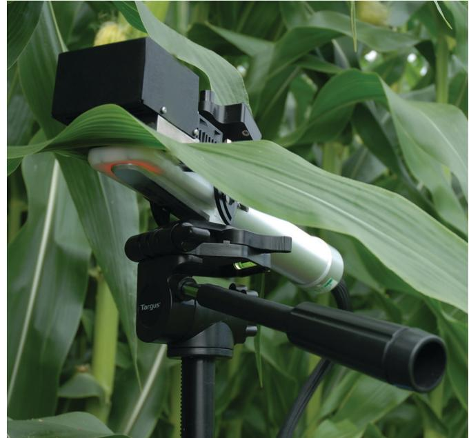
Some considerations are the leaf temperature relative to the ambient outside temperature, the light level, the flow rate through the cuvette and leaf area exposed, and the magnitude of stomatal conductance. There are relatively few circumstances where one can measure leaf gas exchange at VPD lower than 1.0 kPa (except at low temperatures).
