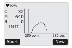
Typically during an injection, the first value will rise quickly and drop back to zero; correspondingly, the value of **M** will increase quickly as the value of **C**, then plateau at a constant value. Once **C** has dropped to 0 ppm (or a very low background value), wait 3-5 seconds to make sure **M** has stabilized and take note of the value. **NOTE:** If using a USB memory stick, the value will automatically be recorded.
