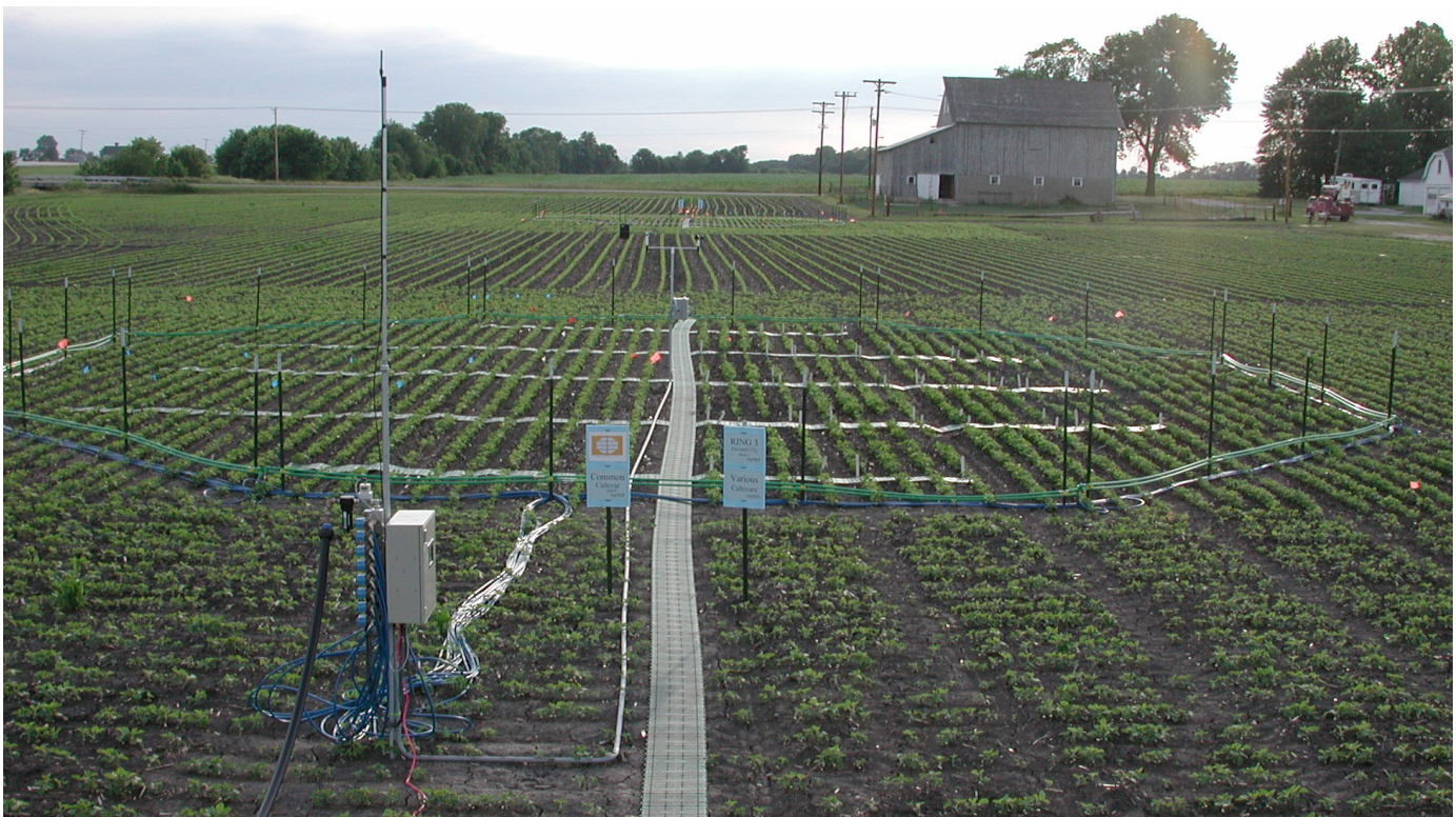
This is an experimental "ring" in a soybean field. The SBA-5 is housed in the enclosure at the center and feeds data to the control box in the foreground. CO 2 is released from the green pipes forming the ring to control CO 2 levels in ambient air.
