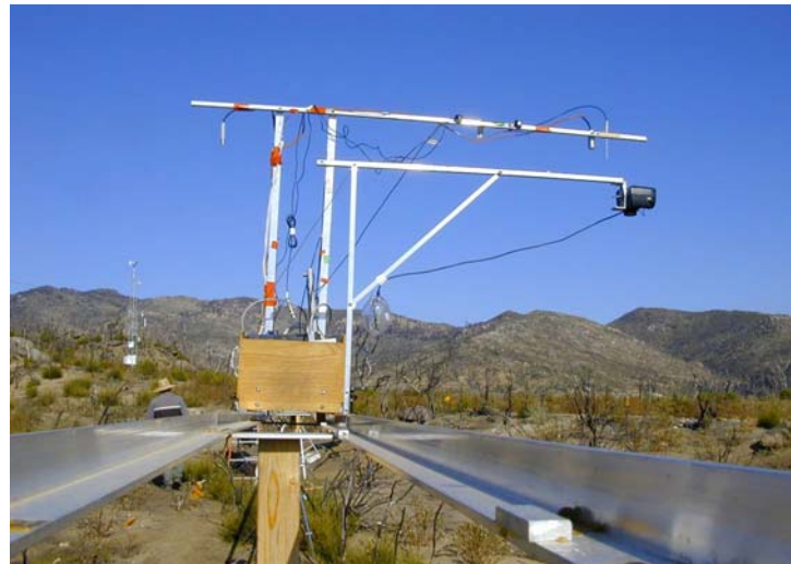
Fig. 1. Schematic and photo of tram system. A UniSpec-DC enables simultaneous sampling of upwelling and downwelling radiation (indicated by cones), providing “on-the-fly” correction for changing sky conditions needed for accurate calculation of spectral reflectance and vegetation indices. Drawing courtesy of Loren MacKinney (Dept. of Biological Sciences, California State University, Los Angeles).
