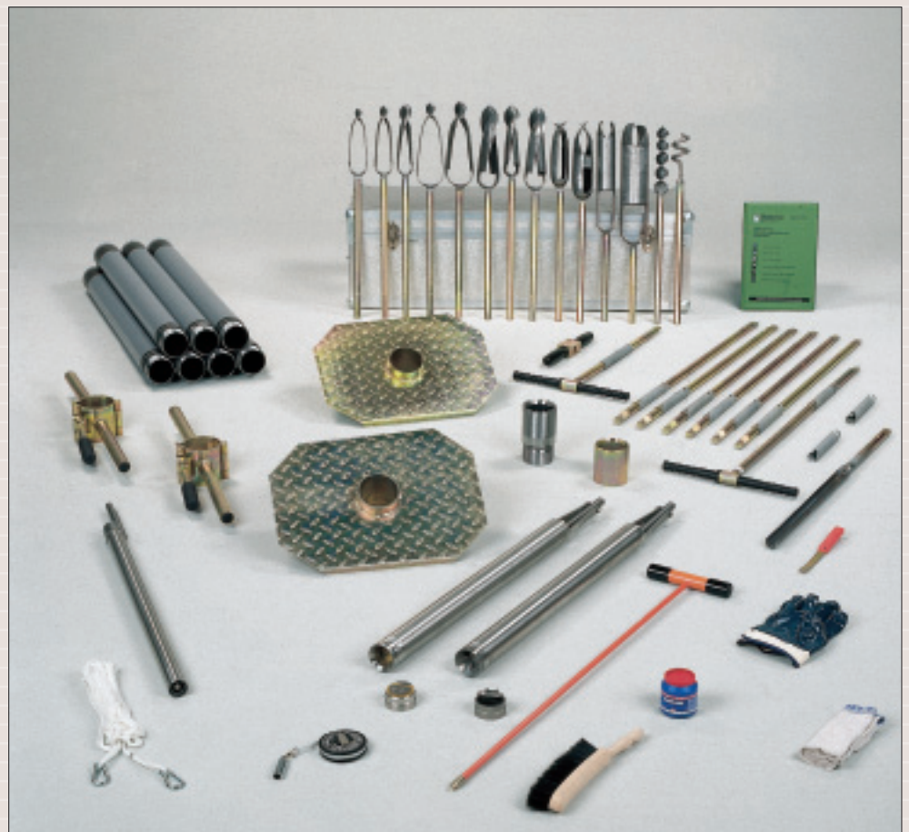
Hand-operated bailer boring auger set
